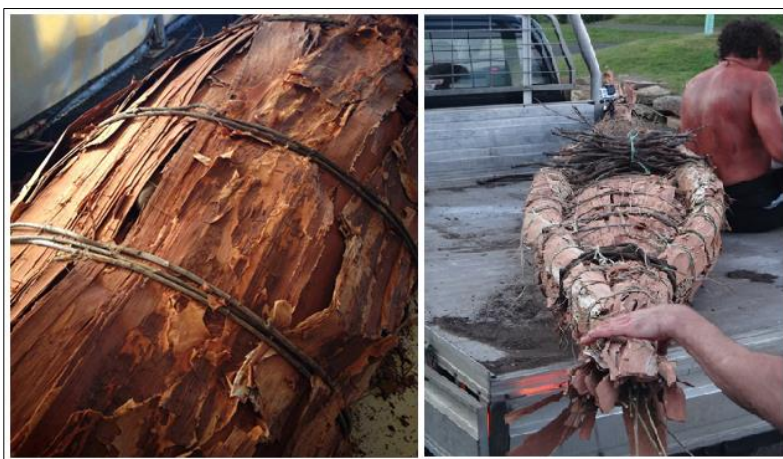
Ningher canoe - ti-tree over juncus reed and tied with bushman's bootstrap. Reprinted with kind permission © F. Hamilton
